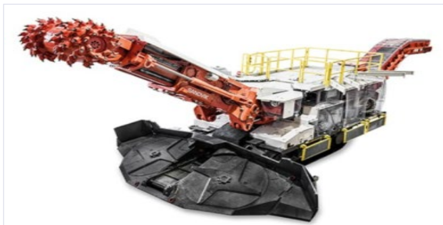
Diagram 23 Example of a Road Header
