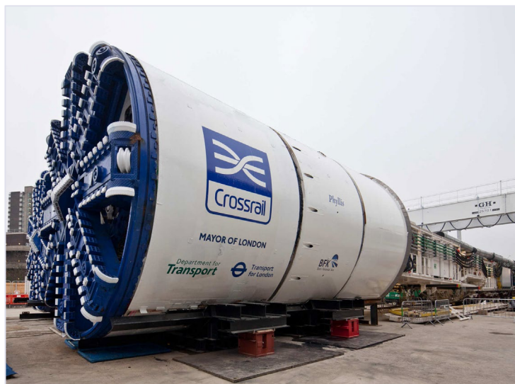
Diagram 24 Example of a TBM
